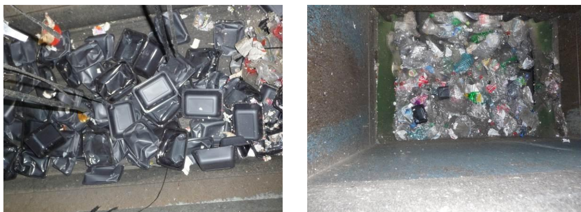
Figure 5: NIR sorting classification to CPET (LHS) and non-CPET (RHS) after single pass.
