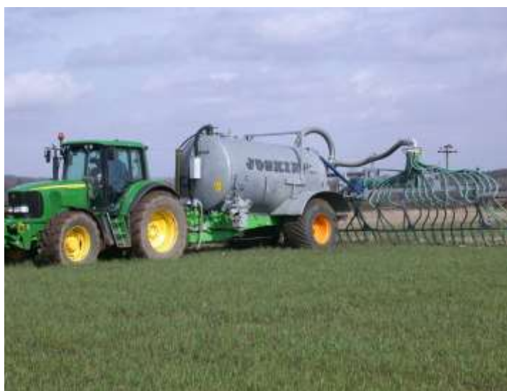
Plate 2.1. ADAS bandspreader application equipment for digestate and slurry.
