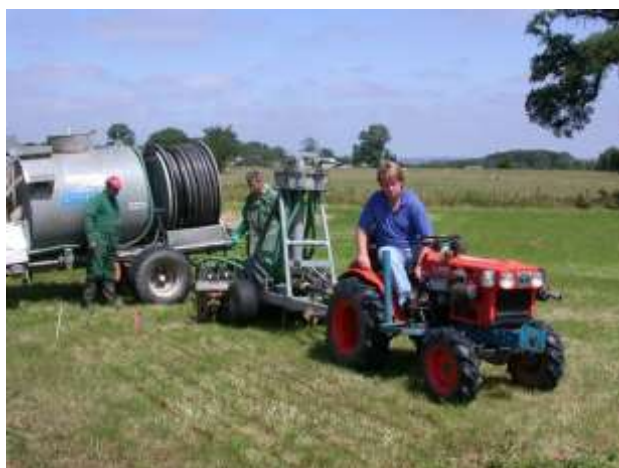
Plate 3.1. Plot application equipment for digestate and slurry.
