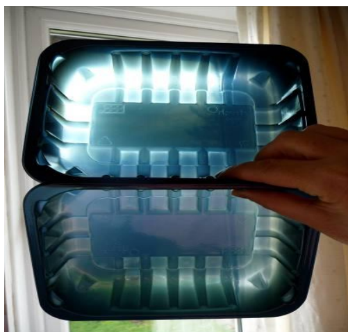
a) APET samples showing difference between 0.5% (top) and 0.8% (bottom) colourant addition rate when held against bright light
