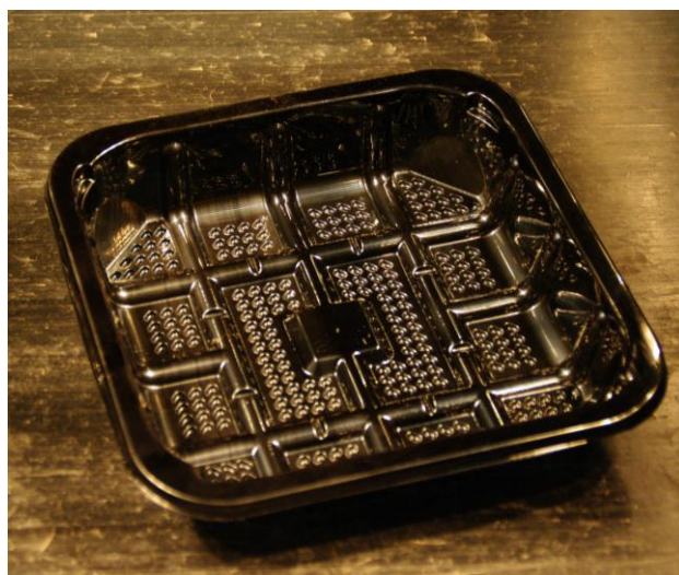
Figure 14. Example of PET tray produced with optimised NIR detectable black liquid colourant from ColorMatrix
