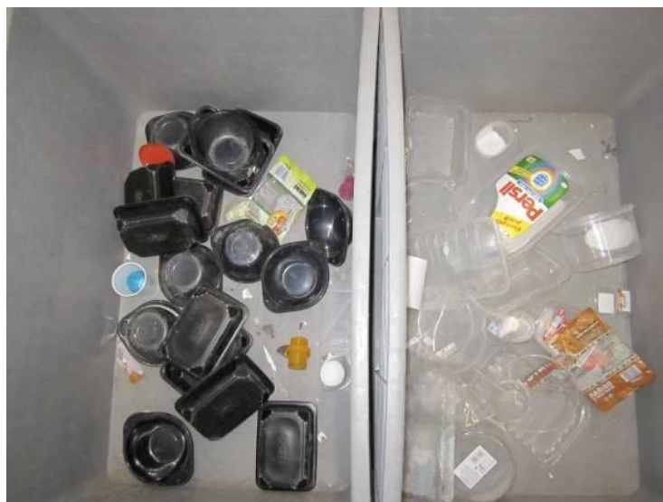
Figure 33. Separation of black PP from clear PP
