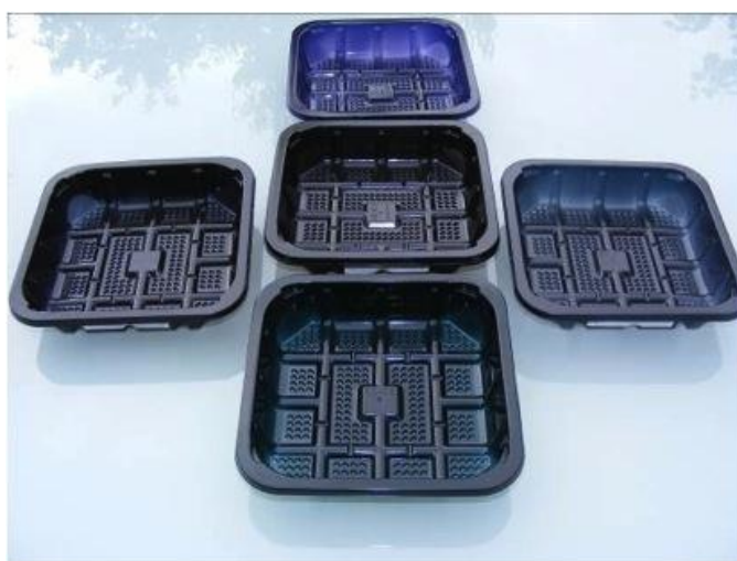
Figure 12. Example of some of the PP trays manufactured with the colourants. A number of the trays were found to have acceptable black finish while others showed shades of dark brown, dark green and blue/purple.
