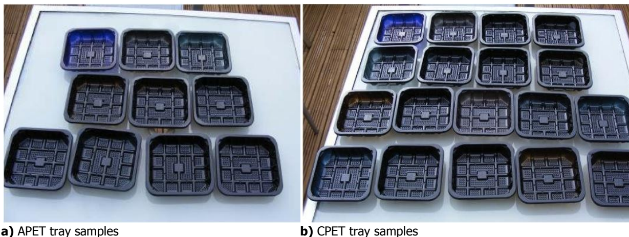
Figure 13. Example of some of the APET and CPET trays manufactured with the colourants
