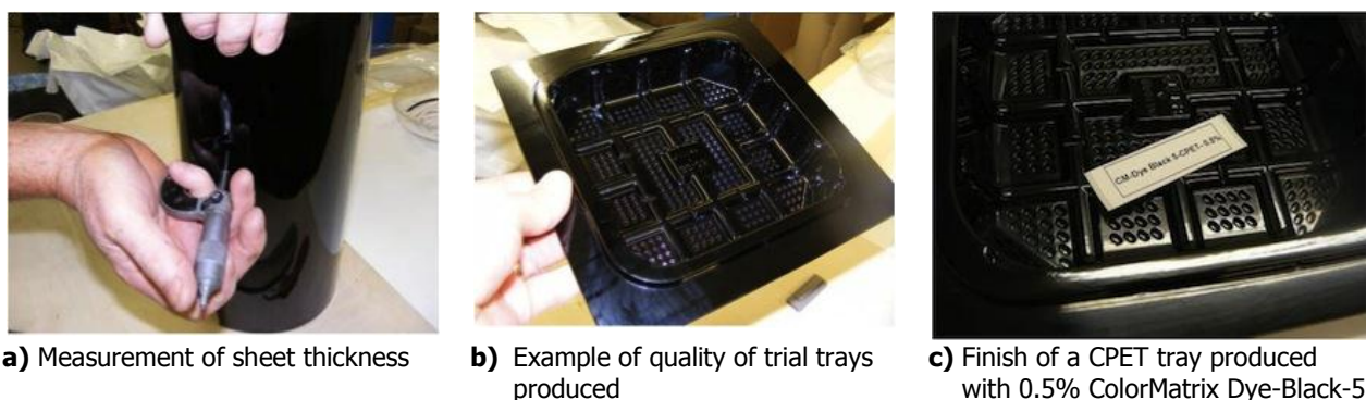
Figure 11. Measurement of extruded sheet and examples of optimised colourants in thermoformed trays
