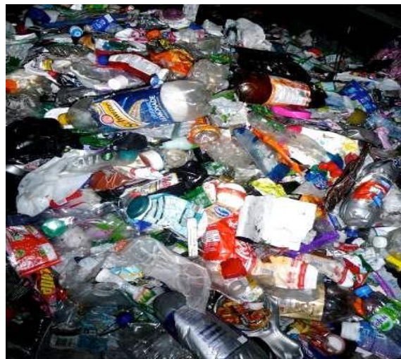
d) Residue "rests" bunker showing no loss of NIR detectable black PET
