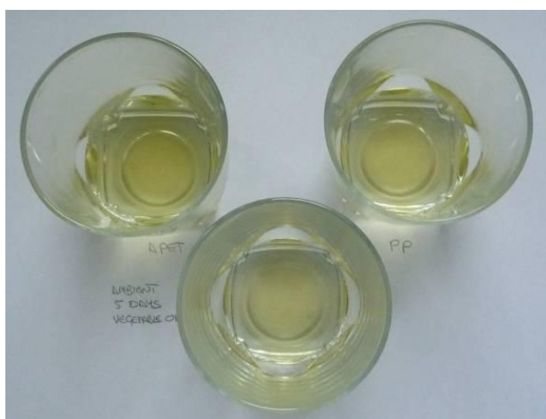
Figure 22. Oil samples showing no colour migration from APET sample with ColorMatrix Dye Black-5 (left), the control sample (bottom) and the PP sample with Colour Tone IRR 95530 (right) after storage for five days under ambient conditions (20 – 25 °C)
