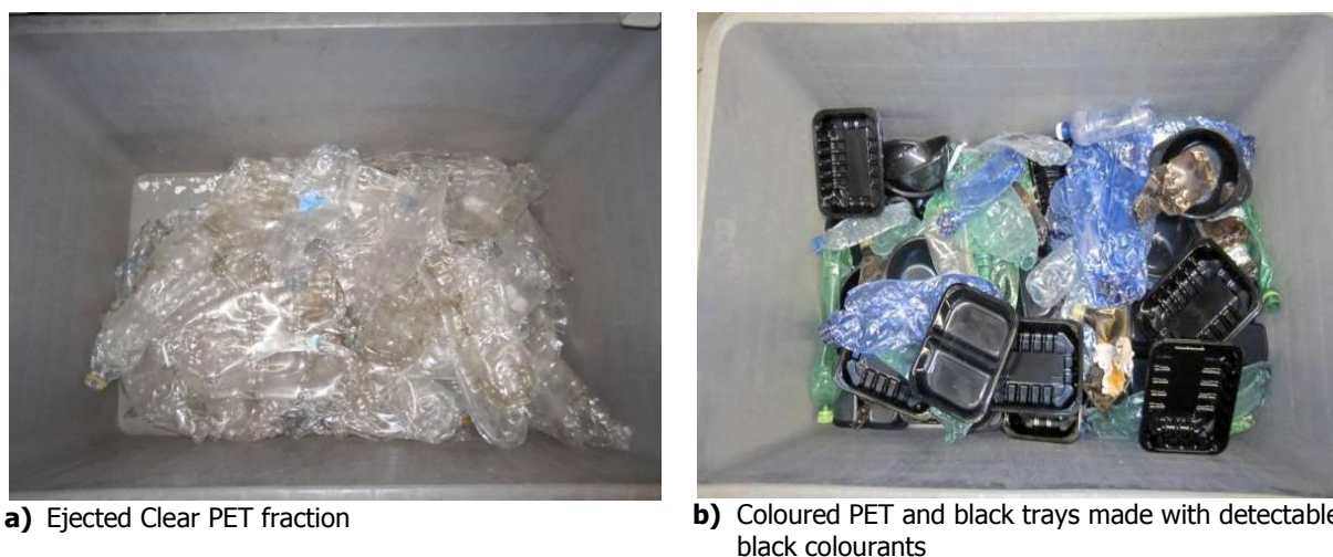
Figure 32. Images of sort bins after TITECH detector was optimised to distinguish black from clear PET
