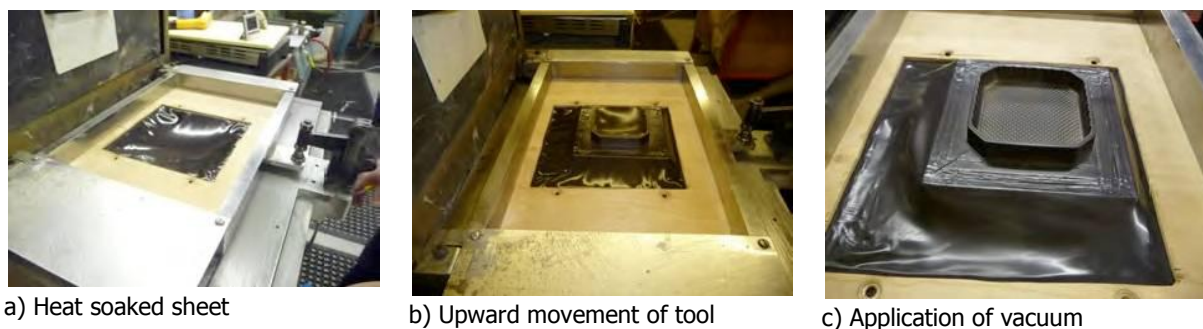
Figure 10. Thermoforming cycle for production of sample trays
