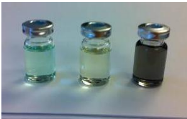
Figure 21. Colour migration into oil from CPET trays after 30 minutes at 180 °C showing the Colour Tone IRR 95530 sample (left) the control sample (middle) and the ColorMatrix Dye Black-5 sample (right)
