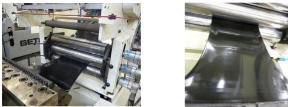
Figure 9. Example of sheet extrusion trials at Brunel University using alternative black colourants
