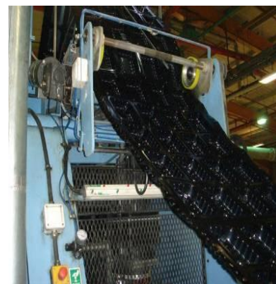
c) Black APET trays being thermoformed at LINPAC Packaging
