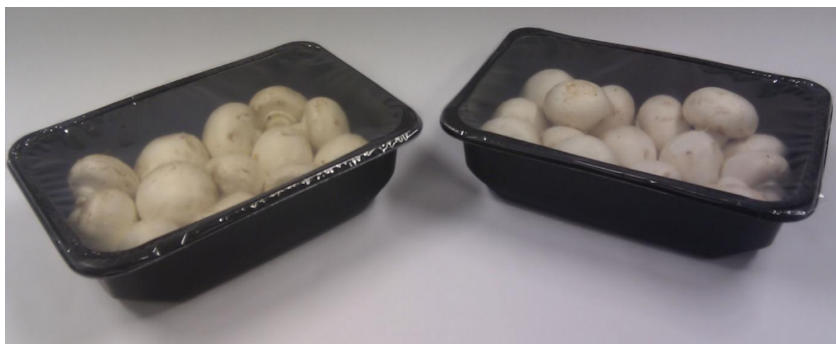
Figure 26. The images below are from the filling and sealing trials completed at Sharp Interpak (the photograph shows 2 punnets, the IRR is on the left side)
