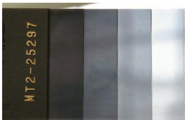
Figure 15. Sample of PP plaque obtained during the development of an alternative black pigment showing low tint strength in thin sections. The thickness of the steps from left to right: 3mm, 2mm, 1.5mm, 1mm, 0.5mm
