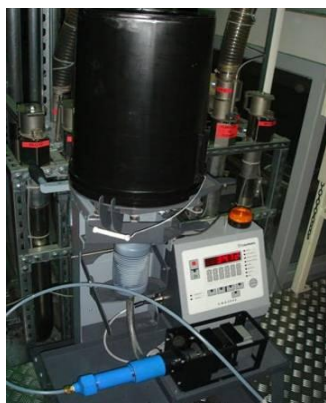
a) Liquid colourant dosing unit for the Dye Black-5 colourant supplied by ColorMatrix
