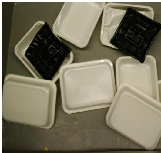
b) Commercially available white CPET trays and black CPET trays made with the novel NIR detectable colourants
